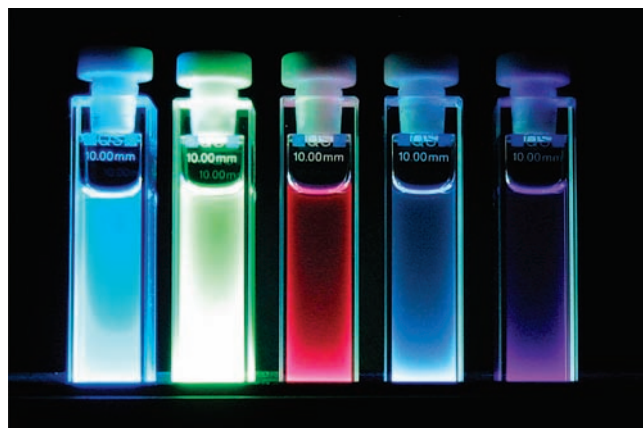
FIGURE 8. Observed emission from Ln(III) cations sensitized by an IAM ligand irradiated with a standard laboratory UV lamp ( \lambda_{\text{ex}} = 365\text{ nm} ). From left to right, ligand only, Tb(III), Eu(III), Dy(III), and Sm(III) complexes.
